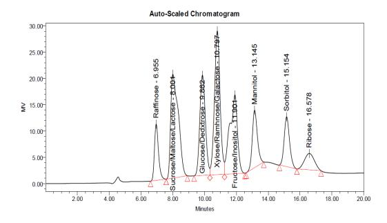
**Figure 6-** HPLC Chromatogram of standards viz. raffinose, sucrose, maltose, lactose, glucose, dextrose, xylose, rhamnose, galactose, fructose, inositol, mannitol, sorbitol and ribose using water as mobile phase.
